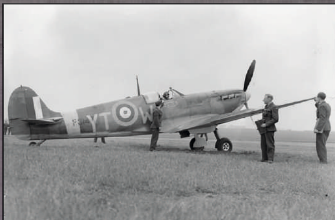
No. 65 Squadron Spitfire Mk.IIa, P8147, at RAF Kirton in Lindsey in the summer of 1941. This aircraft is equipped with a De Havilland 5/39A constant speed propeller. Note the atypical bottom surface painting and fuselage band. Metal ailerons are possible on this aircraft. (photo: Simon Erland)
