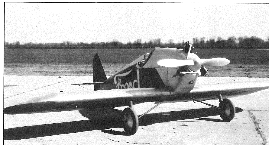
Full-span version during 1927. Note actuating linkage beneath wing and that propeller and spinner appear all one color. Photo from Underwood/Collinge collection.
