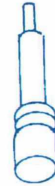
I Band Transponder - these have now been removed from 'Grey Whale' HAR.3s, but are present on all other UK variants.
