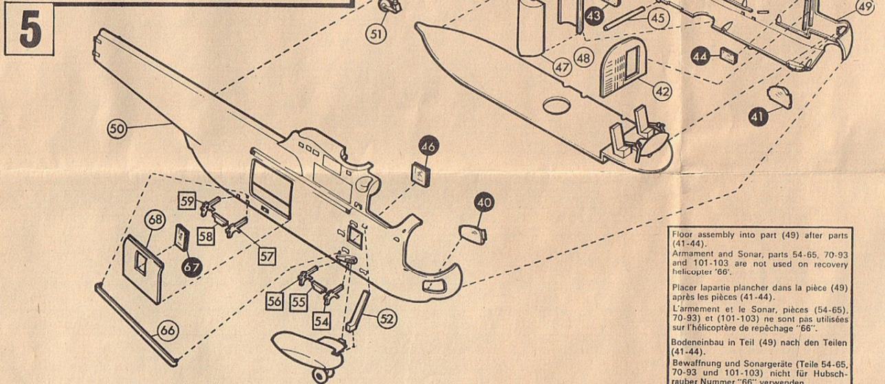
Floor assembly into part (49) after parts (41-44).
