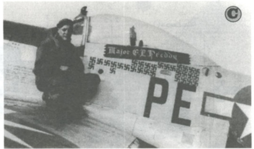
Assistant Crew Chief Sgt. Deigman on the wing of Cripes (fourth) in late October 1944. Note the flare port between the bottom two swastikas, the fuel filler cap, and the location of the Black ID stripe under the fuselage star.
