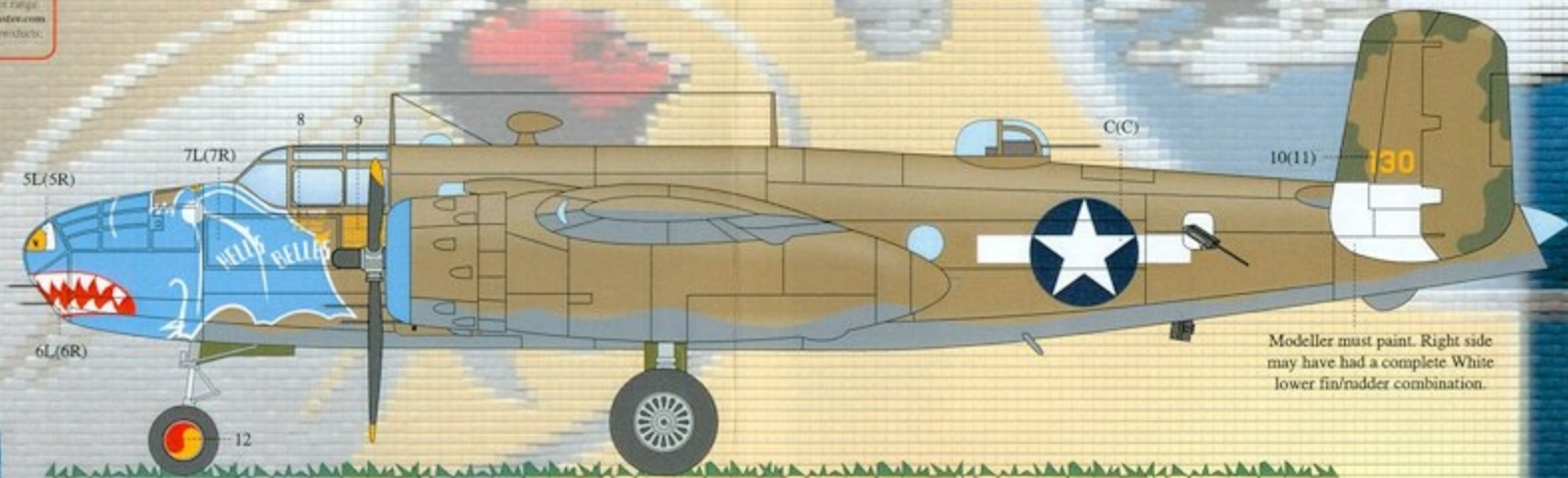
"Hell's Belles", B-25D-1, #41-30019. 499th Bombardment Squadron, 345th Bomb Group, Port Moresby, November 1943. Upper surfaces Olive Drab with Medium Green splotching on wings and tail surfaces, Neutral Gray undersides. Note replacement port rudder, leaving only a partial serial number. Medium blue cowl rings. Note plexiglas tail cone has been cut away, most likely to provide for fitting an additional hand-held machine gun. Aircraft had .50 caliber machine guns in small rear fuselage windows. Mask your canopy. Spray paint your Medium Blue color. Mask your cowling ring. Transfer the masking template to masking paper or whatever masking you use. Cut it and apply to the nose section following the instructions. Paint your Olive Drab and Neutral Gray colors. Remove the masking over the Medium Blue color. (Not your transparencies). Make sure the colors are glossy. Use your decal 7L and 7R to trim the Blue and the Olive Drab/Neutral Gray colors.
