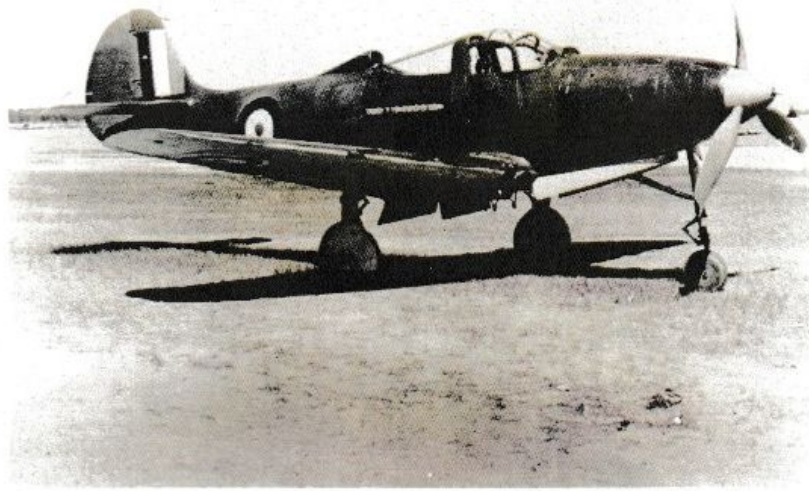
A53-unknown Number 2. This aircraft is fitted with an anodised aluminium propeller which appears to be devoid of the yellow painted tips. The spinner appears to be either a replacement that has yet to be painted or possibly may have been finished in RAAF Sky Blue.
