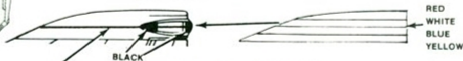
CENTER LINE BETWEEN WHITE AND BLUE STRIPE ON CENTERLINE OF RHAW ANTENNA.
