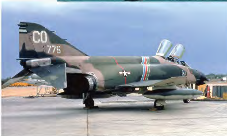
F-4D-32-MC 66-8775 in her factory paint, again illustrating the glossy black translating ring and inboard stabs.
