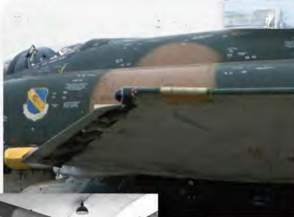
Left: the left wing tip light on F-4E-54-MC 72-1484 showing what we believe to be the early configuration of the slatted wing tip light. Note the brownish frame around the light.
