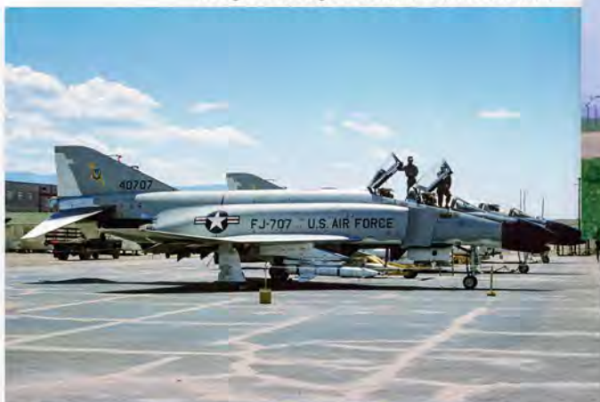
F-4C 64-0707 on display. Note the plethora of white inspection dots, and the very visible "pie wedge" of Corogard above the exhaust nozzle.
