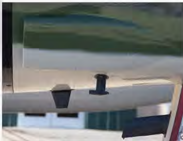
A retired F-4C showing the standard TAT probe position below the port ECS inlet fairing.
