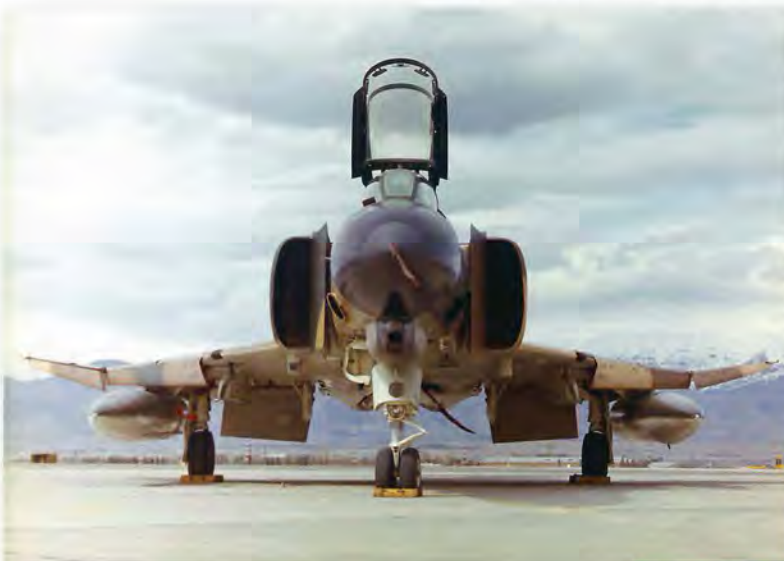
Above: Iran's initial F-4E deliveries were -46 and -47-MC blocks with FY69 USAF serials, delivered between Mar and Nov 71. As such, these were all hard wing aircraft, and survivors were upgraded with slats in 1973-74. Many continue in service with the IRIAF today after having served for over 50 years and participated in at least two wars - the Dhofar War of 1973-76 in Oman and the Iran-Iraq war of 1980-88.
