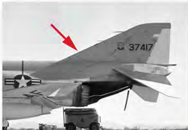
F-4C-15-MC 63-7417 which first flew on 27 Sep 63, still with the original style TAT fitted into the fin leading edge.
