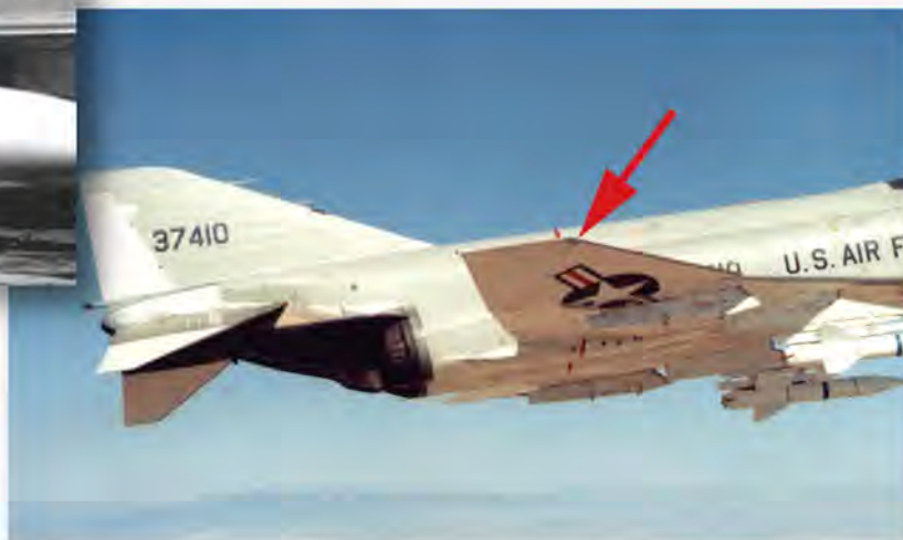
Right: F-4C-15-MC 63-7410 showing the flush style lights.
