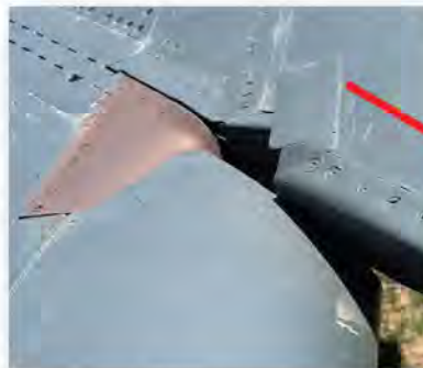
The left wing BLC exhaust on an RF-4C. This detail is identical on all hard wing F-4 variants (F-4B/C/D/early E/J/RF-4B/C/E).
