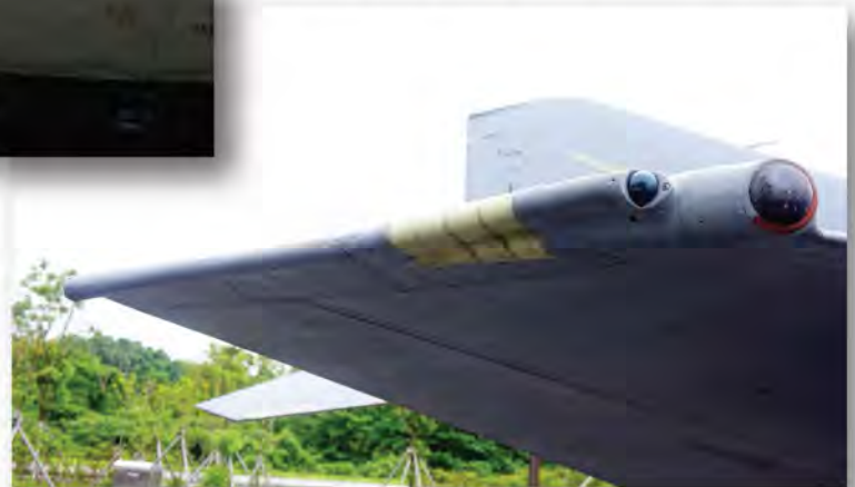
Left: a shot of an IDF hard wing F-4E with the narrow black framing around the light strips. These were often seen mixed with unframed light strips on the tail on the depot installed lights.
