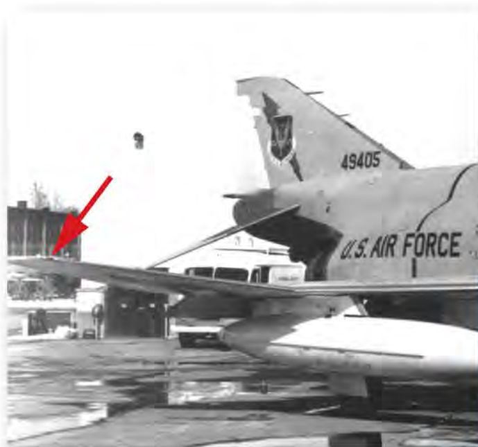
Left: F4H-1 149405 Block 9, alias F-110A is seen shortly after roll out in Jan 62. She has the original flush style nav lights.
