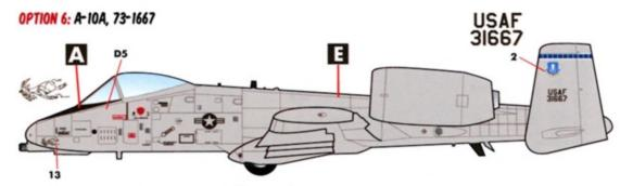
73-1667 WAS THE FIRST A-10 TO BE PAINTED IN "MASK 10A" PAINT. ACCORDING TO PRI-FLY, THIS COLOR LOOKS CLOSE TO FS36424 IN MOST LIGHTING CONDITIONS. NOTE BLACK MAINTENANCE STENCILLING AND NATIONAL INSIGNIA, BUT WITH FULL COLOR EJECTION SEAT TRIANGLE AND LADDER WARNING MARKING. EDWARDS TAIL BAND ON THE OUTSIDE OF FINS.
