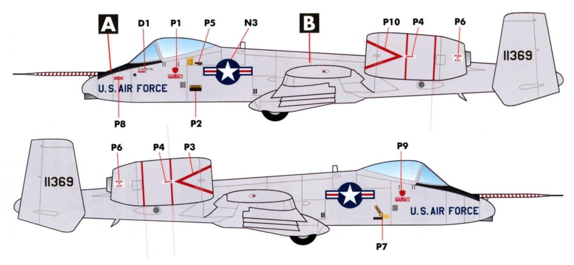
THE FIRST A-10 PROTOTYPE WAS DIFFERENT FROM THE PRODUCTION VERSION IN MANY WAYS. NOTE THE PROFILE OF THE VERTICAL STABILIZER, THE 20MM VULCAN GUN IN THE NOSE, AND DIFFERENT PANEL LINES. YOU WILL NEED TO MODIFY YOUR BASE KIT TO REFLECT THESE DIFFERENCES.
