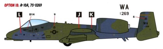
THE CAMOUFLAGE SCHEME THAT WAS APPLIED TO THIS AIRCRAFT LATER BECAME THE BASIS OF THE STANDARD "EUROPEAN ONE" CAMOUFLAGE SCHEME FOR THE A-10. NOTE BLACK MAINTENANCE STENCILLING AND NATIONAL INSIGNIA.
