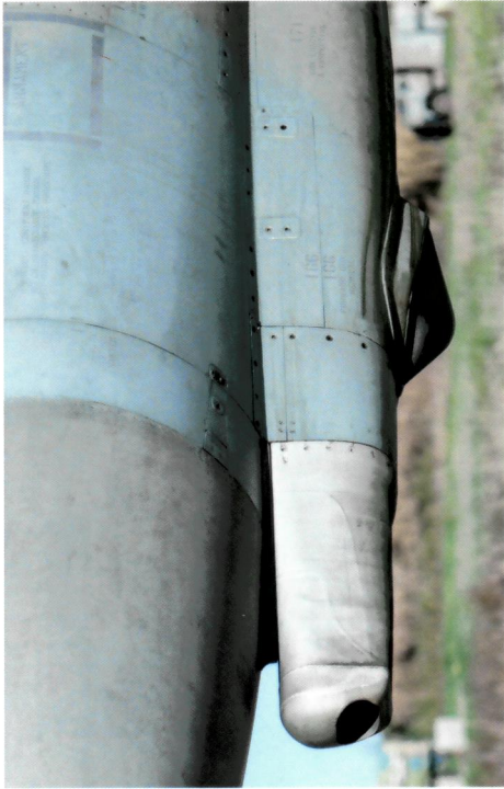
Shape and place of front sensor on gun bay
