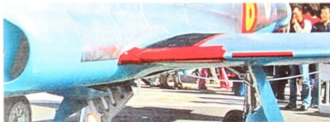
Typical red "NO STEP" area at wing root leading edge.
