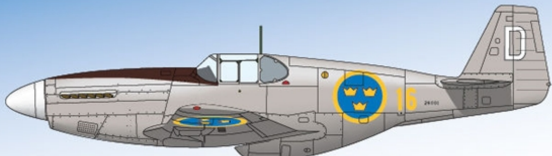
J 26, 26001, white David F16 Uppsala. In the later marking with natural metal fuselage and with wings, elevators and rudder painted in Silver dope. Black stencils and walkways on both wings, during the last period of the angled design.
