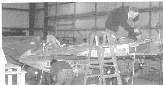
Workers are taking Glacier Girl apart they can start the 10 year restoration. They found that every part of the plane was damaged but about 80% of the plane was saved. 약 10% 정도 복원작업이 진행된 상태. 기체의 거의 모든 부분에서 손상이 발견되긴 했으나, 전체의 약 80% 정도는 사용 가능했다.
